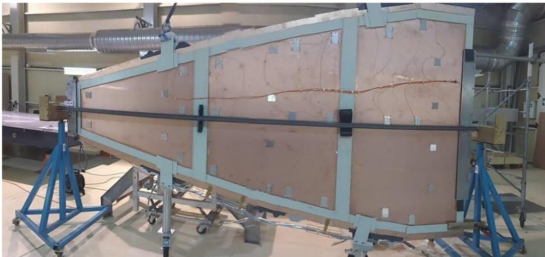
**Figure 4: Three sTGC quadruplets assembled in a wedge, with alignment fibers routed on the surface**
