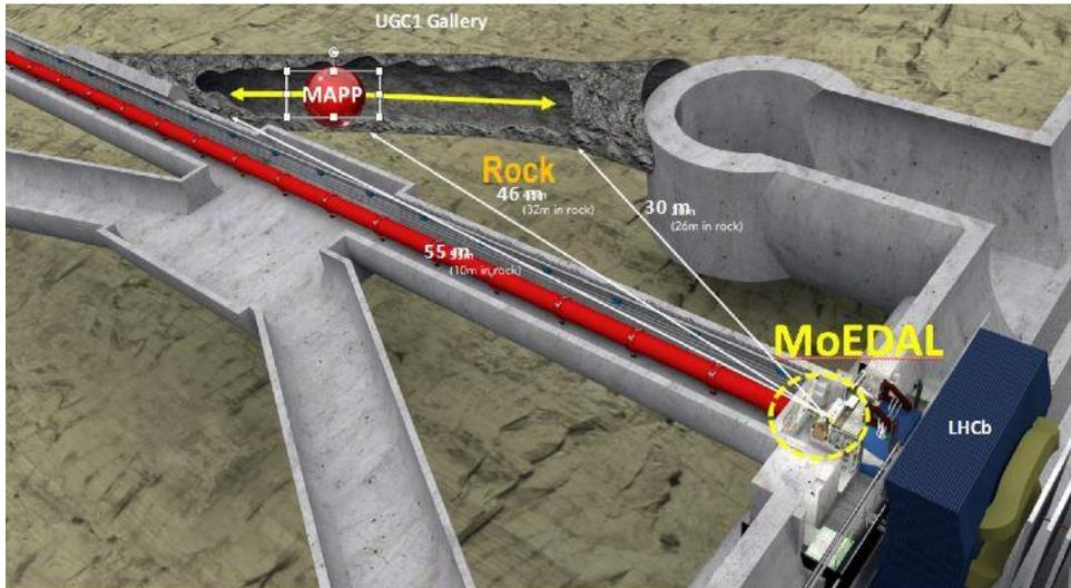
**Figure 4. The MoEDAL MAPP sub-detector deployed in the UGC1 gallery in the vicinity of IP8.**
