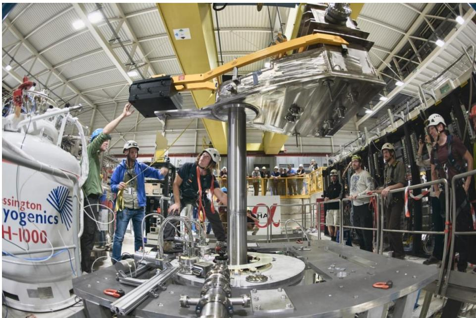
**Figure 3: Insertion of the detector assembly (radial TPC and barrel scintillator) into the main ALPHA-g solenoid**
