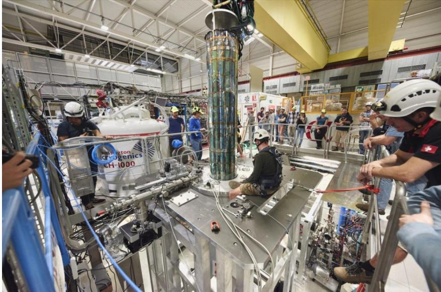
**Figure 2: Insertion of the ALPHA-g cryostat with the antihydrogen trap magnets into the centre of the main solenoid, radial TPC and barrel scintillator.**
