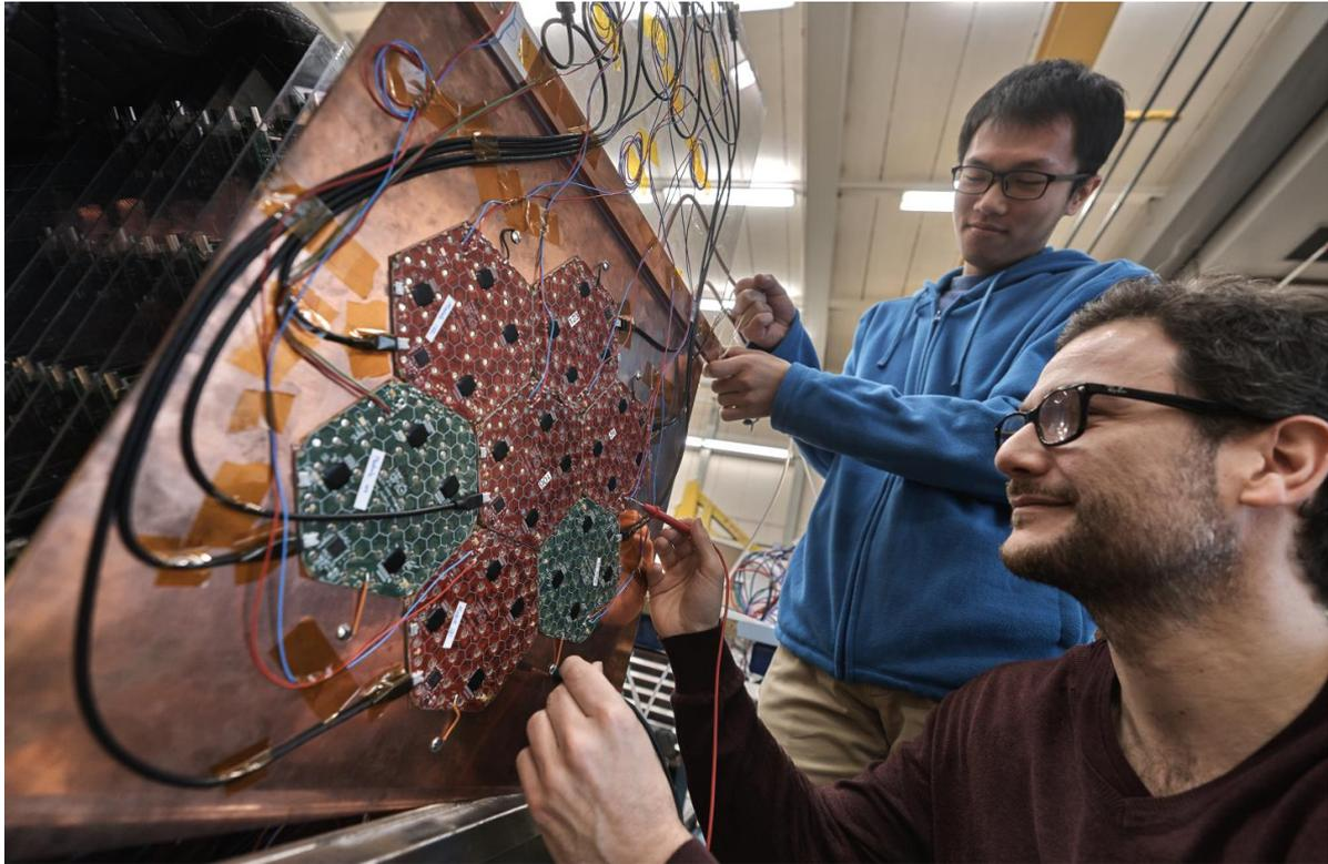
**Figure 1: Ongoing tests on the modules of the High Granularity Calorimeter. Intense R&D is foreseen during LS2 to ensure that the new detector will be ready for installation during LS3.**
