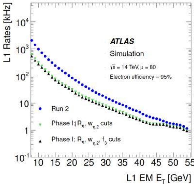
**Figure 2: The foreseen improvement of the ability to reject jets and preserve electron and photons by the scheduled upgrade of the LAr electromagnetic calorimeter.**
