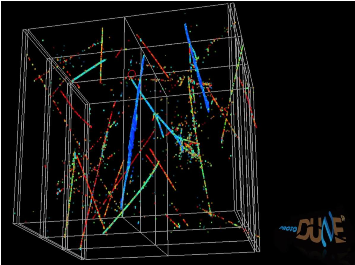
Figure 3: A reconstructed test-beam  $\pi^+$  (entering the TPC from the red circle) interacting inside ProtoDUNE-SP with a number of coincident cosmic ray muons.
