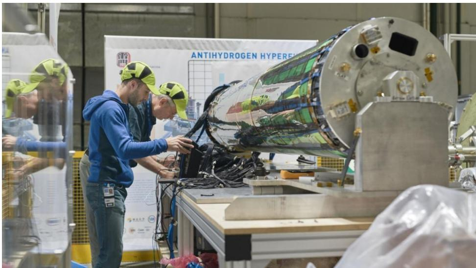
**Figure 1: The Barrel Scintillator for ALPHA-g Experiment is composed of 64 trapezoidal scintillating bars arranged in a barrel shape. Each bar is readout at each end with SiPM sensors for a total of 128 channels.**
