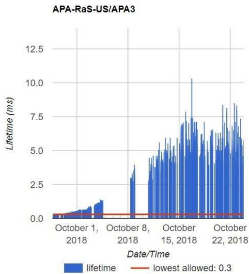
Figure 2a: Electron lifetime estimated from the semi-offline data quality monitors using cosmic-ray muons (left)
