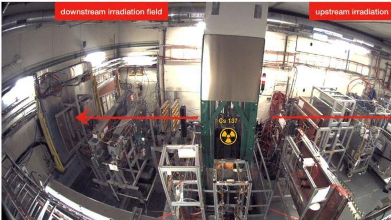
**Fig.2 – GIF<sup>++</sup> irradiation bunker during October Muon beam time 2018. Up to 11 different setups – often composed of multiple chambers – could be hosted along the muon beam, while several other experiments could continue to use only the irradiator.**
