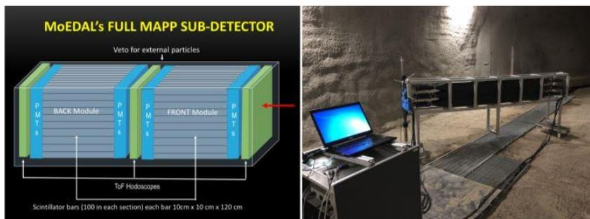
**Figure 5. (Left) A sketch of the proposed MAPP sub-detector. (Right) A photograph of the MAPP prototype deployed in the UGC1 gallery.**
