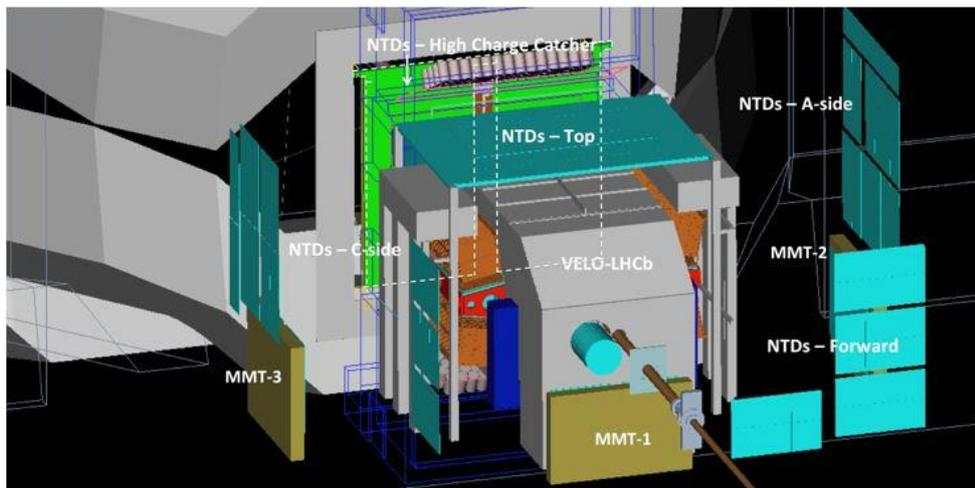
**Figure 1. A visualization of the Geant4 simulation of the MoEDAL experiment, represented using Geant4's PANORAMIX.**
