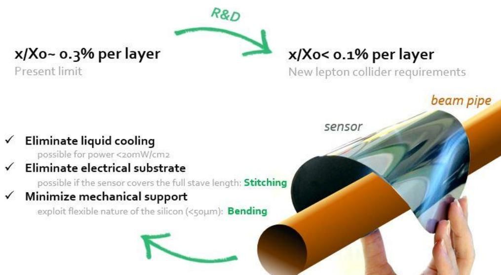
**Figure 3: future vertex detectors aim to unprecedented minimum material budget which call for R&D on new sensor technologies and cooling solutions.**
