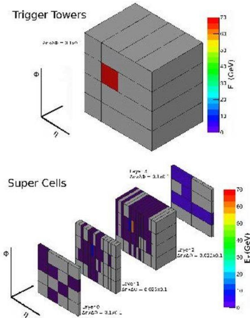
**Figure 1: The so-called trigger towers in which information is stored by the ATLAS electromagnetic calorimeter.**
