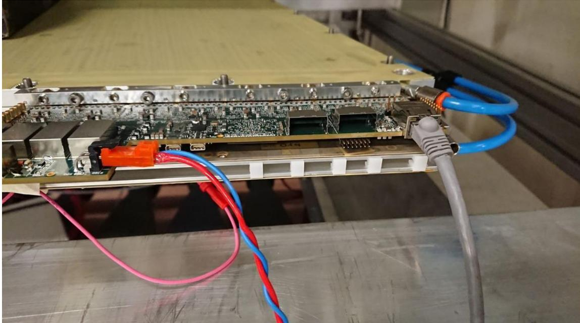
**Figure 5: A Micromegas test Front-end board mounted on the chamber**
