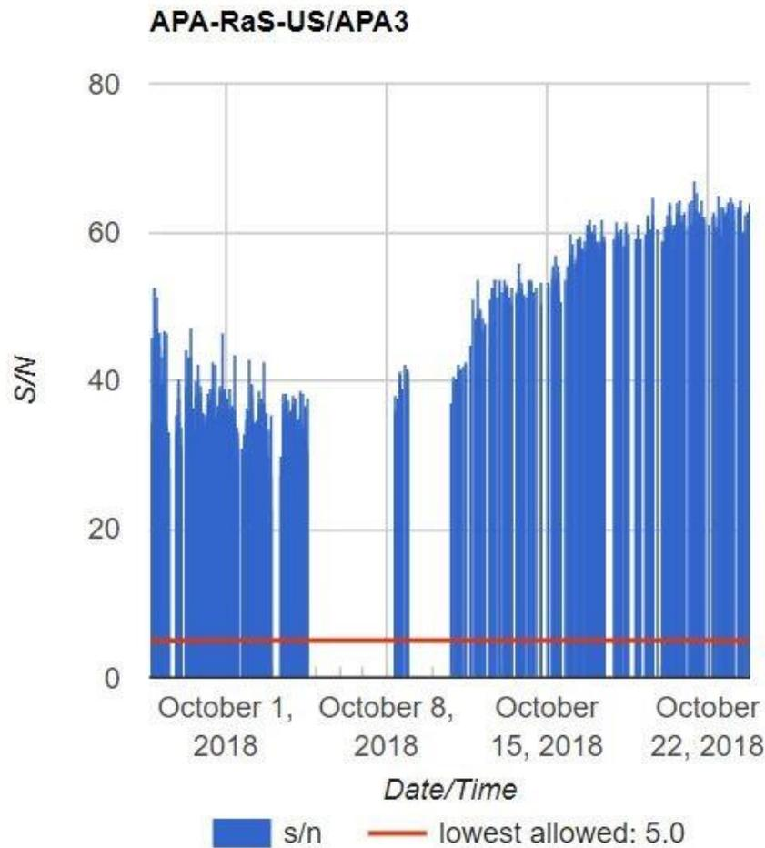
Figure 2b: Signal-to-noise ratio estimated from the semi-offline data quality monitors using cosmic-ray muons (right).
